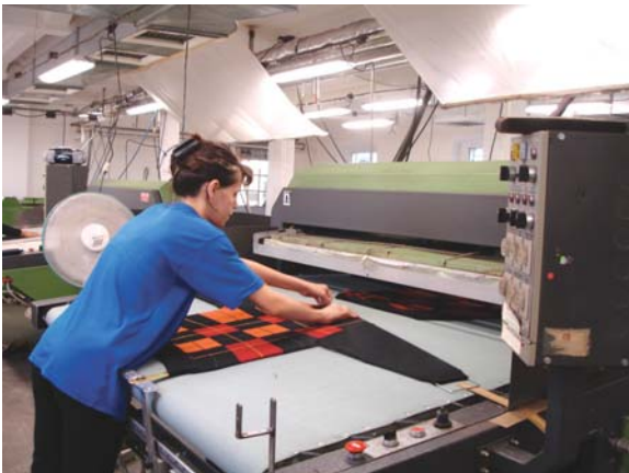
Framing the sweater prior to automatic streaming and finishing - Brod and Co
